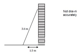
To be safe to use, the base of this ladder must be 1.5 m away from the wall. The ladder is also placed on flat horizontal ground.
